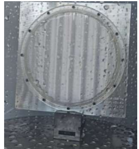
Test Under Water Jet
