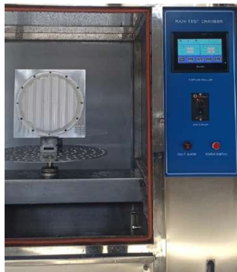
Test Under Water Jet
