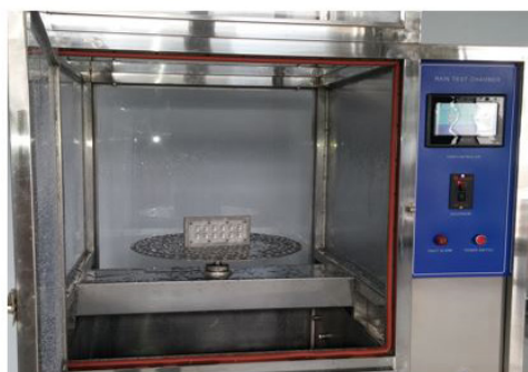
Testing under water jet
