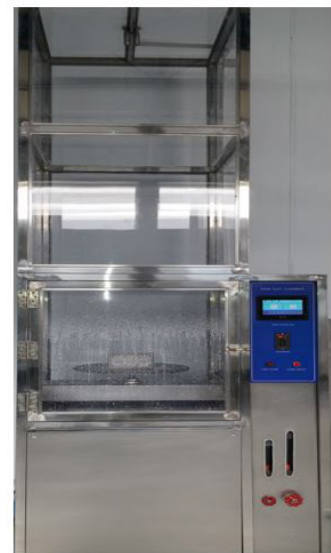
Testing under water jet
