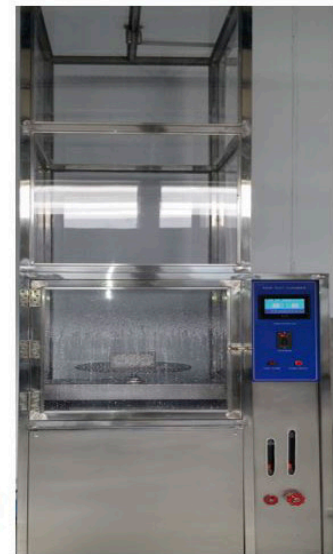
Testing under water jet
