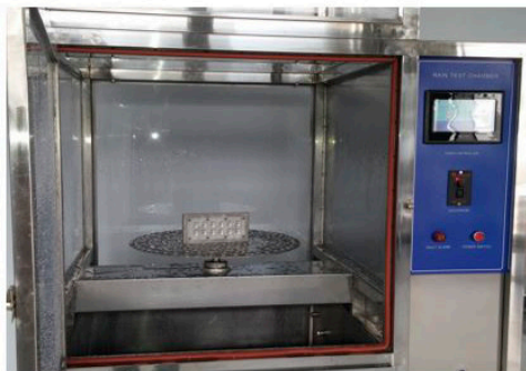
Testing under water jet
