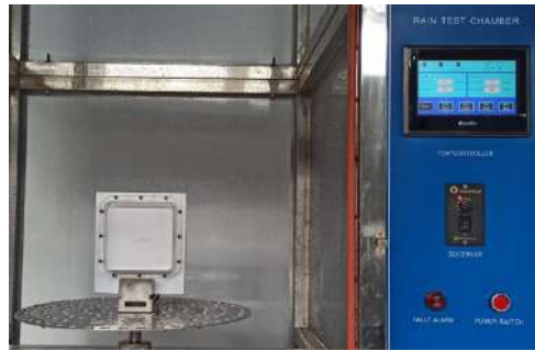
Test Under Water Jet
