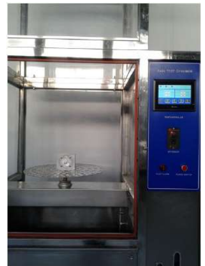
Testing under water jet
