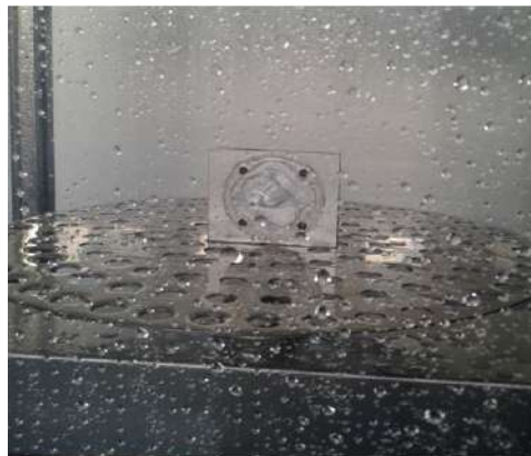
Testing under water jet
