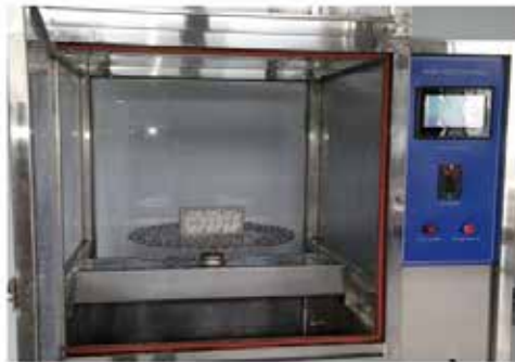
Testing under water jet
