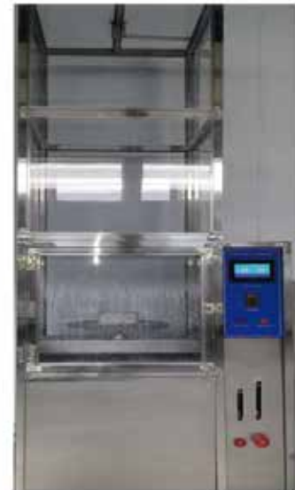
Testing under water jet
